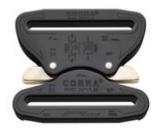
The COBRA® PRO STYLE is a buckle that meets the highest safety requirements for its users, as it can only be opened when released by pressing both clips at the same time. The locking mechanism thereby allows easy engagement of the interlocking components, which is confirmed by a distinct clicking sound. One-sided locking is nearly impossible.
