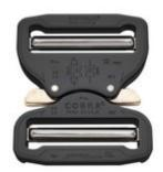
The COBRA® PRO STYLE is a buckle that meets the highest safety requirements for its users, as it can only be opened when released by pressing both clips at the same time. The locking mechanism thereby allows easy engagement of the interlocking components, which is confirmed by a distinct clicking sound. One-sided locking is nearly impossible.
