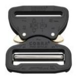
The COBRA® PRO STYLE is a buckle that meets the highest safety requirements for its users, as it can only be opened when released by pressing both clips at the same time. The locking mechanism thereby allows easy engagement of the interlocking components, which is confirmed by a distinct clicking sound. One-sided locking is nearly impossible.
